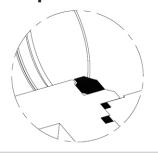
Detail of Protected seat & encapsulated body seal design. Isolates & protects both seats and seals from flow path. Helps to prevent cold flow.
